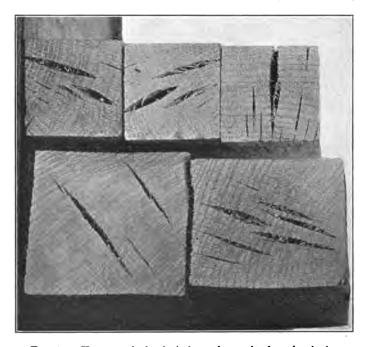
Fig. 66.—Honeycombed oak timbers, the result of casehardening.
